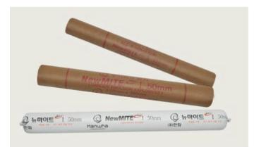
*NewMITE*<sup>™</sup> *Plus* is available in two packaging types, paper cartridge or film depending on the customer's preference and use. In particular, the paper cartridge packed *NewMITE*<sup>™</sup> *Plus* is easy to load horizontally as it has the same compound phase as dynamite.
